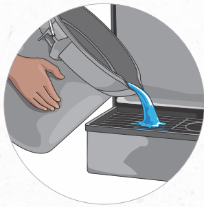
1 Pour 1/2 gallon of approved sanitizer over cup rest and down the drip pan drain
