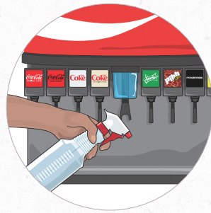
1 Spray down surface of the dispenser (valves, levers, & sides)
