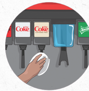
9 Wipe the lower valve body and lever dry with a clean cloth
