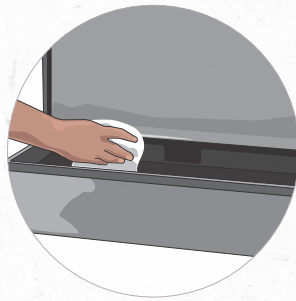
2 Remove rack, wipe down the drip pan with a clean cloth and approved sanitizer
