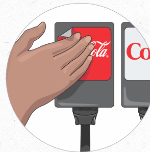
Check product valve decals and replace, if necessary
